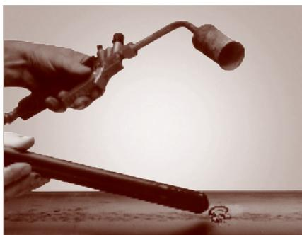
Installation is done with a standard gas torch. After eliminating all sharp edges, cleaning and preheating, PERP-MELT-STICK is heated above the damaged area until becoming glossy. No filler is required. The molten adhesive is spread onto the scratches, forming a tight bond with the substrate. After cool down, the hardening adhesive is smoothed flush with the PE line coating using a paint scraper.
